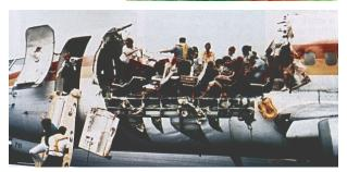
Fig.2. The need to control far-from equilibrium behavior. Top: Turbulent airflow produced by the wingtips of a small airplane (visualized by red smoke). Bottom: Disastrous effect of materials fatigue and eventual fracture.
