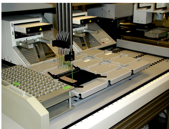
Robotic preparation of MALDI mass spectrometry samples on a sample carrier.
